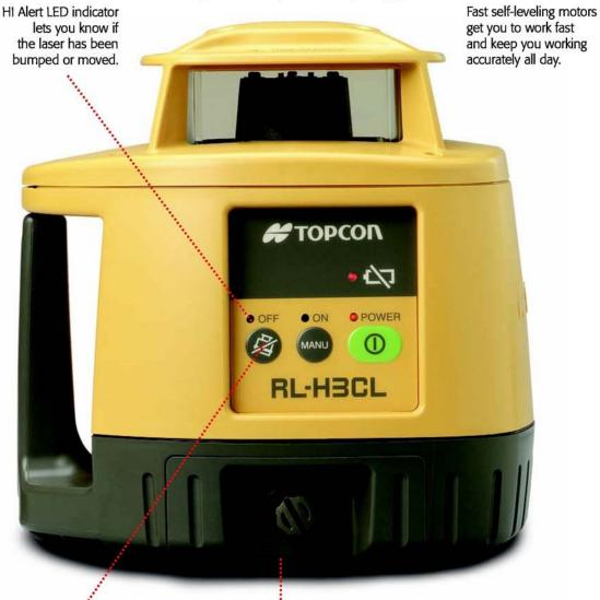
HI alert can be turned off when using a slope block or matching a slope. Sealed battery compartment accepts 4 "C" size alkaline batteries.
